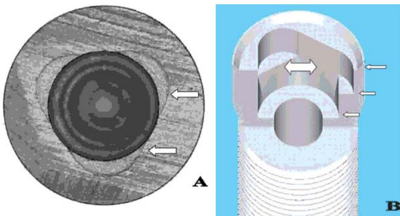
Figure 4. Optical micrographs (x50) of BTLock implant as transversal cross-section (A) and autoCAD design (B). Asymmetric double-triangulated 3-levelled internal connection as a guaranty of high stability between fixture, pillar and abutment and anti-rotational stability is visible
