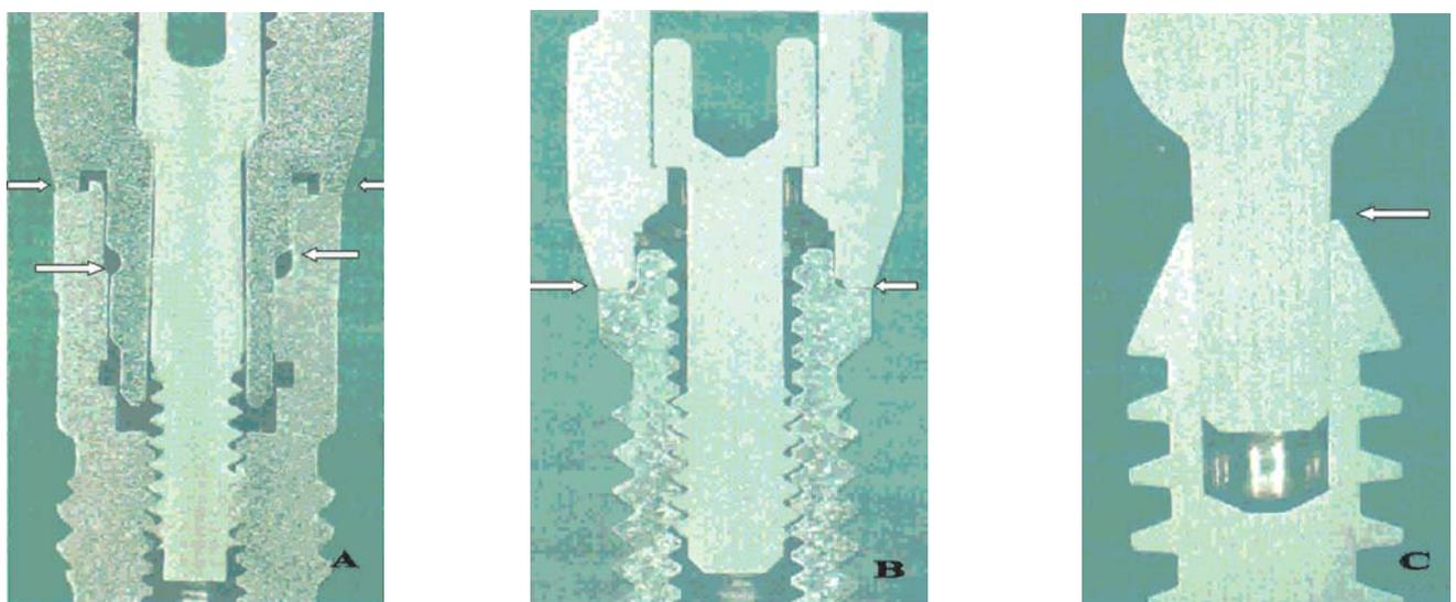
Figure 5. Optical micrographs (x50) of 3 representative classes of commercially available implants: A) with internal connection (arrows show symmetric 1-level closure); B) with external hex connection (arrows show symmetric 1-level closure); C) conical seal connection
